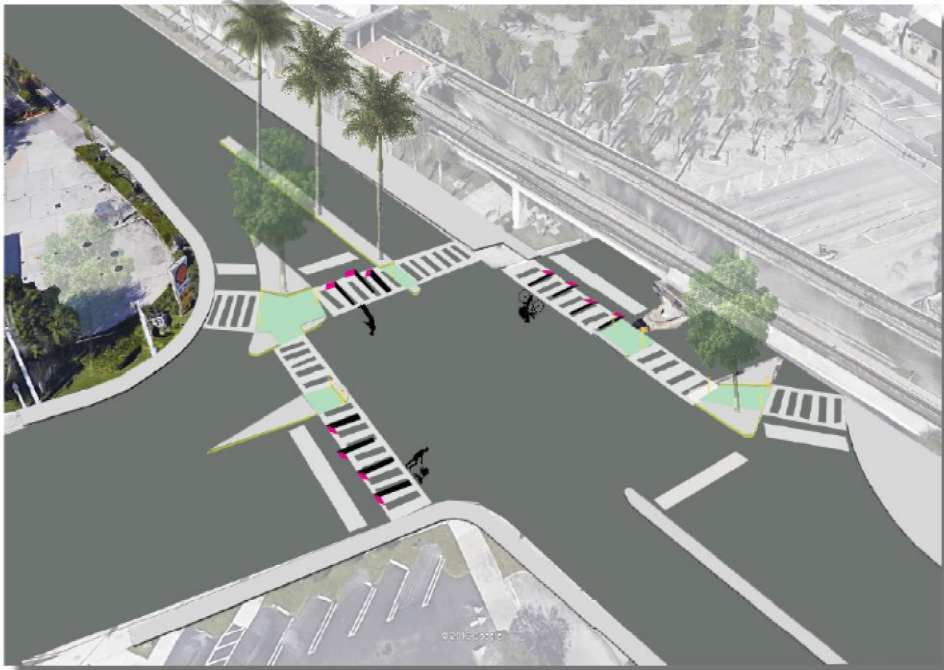
Rest islands and on-street graphics for safer pedestrian crossings
